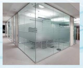
Glass partition is a concept to divide the available large space in to convenient and desired partitions. Various partition angels are achieved with the glass partition concept with the help of toughened glass. The process of glass partition is designed by architecture based on the purpose and convenient of the end users. Large scopes of commercial and residential spaces can be segments as glass partition.
